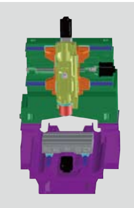
Thermally symmetric structure Equal left-right construction permits straightforward thermal distortion
